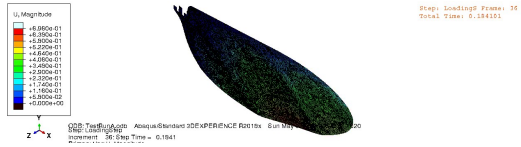
Fig. 15. Screenshot of last increment of the static analysis before crashing. This simulation failed at 20% time increment.
