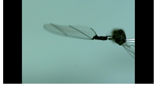
Fig. 4. Frame captured from the static flapping test. Stroke angle measurements are then taken from the videos.
